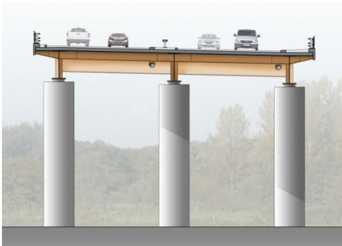
Figure 4-9: Illustrative cross section of the viaduct structure showing the deck and piers
